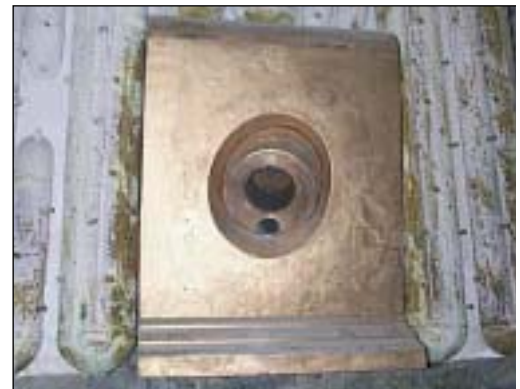
1 Pyrejet burner nozzle viewed from within furnace showing carbon pipe outlet and burner set in water-cooled copper wall tiles
